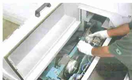
The heavy duty **saw carriage** guarantees maximum stability and very high precision of the cut. The saw carriage is equipped with quick **pneumatic saw blade release**.
