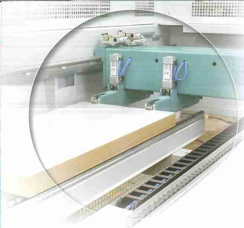
**Electronically controlled pusher** with overhead side guides equipped with pneumatic grippers.
